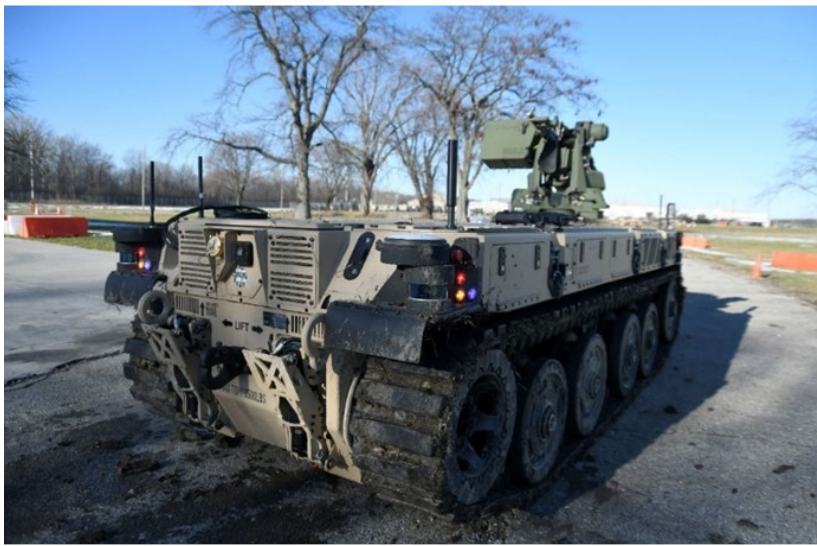
The Robotic Combat Vehicle-Light (RCV-L) experimental prototype is a small, lightweight hybrid-electric unmanned ground combat vehicle that can be transported easily by military aircraft. Its highly versatile common architecture and modular payload features offer a scalable continuum of capabilities that can be adapted to new and emerging threats well into the future.
