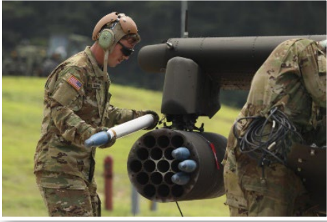
Soldier assigned to 5-17 Air Cavalry Squadron, 2nd Combat Aviation Brigade, 2nd Infantry Division, is seen loading a Hydra 70 missile into the AH-64E Apache Helicopter
